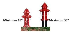
The center of a hose outlet shall be not less than 18 in. or greater than 36 in. above final grade
