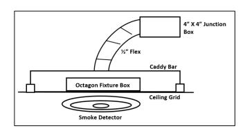
14. Subfloor Smoke Detector Mounting Detail
