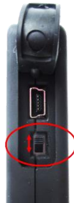
Figure 4-15. FirstVu HD Power Switch (on DVR)
