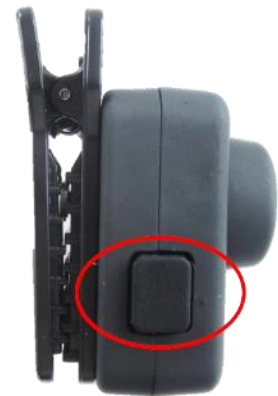
Figure 4-16. FirstVu HD Record Button (on Camera)
