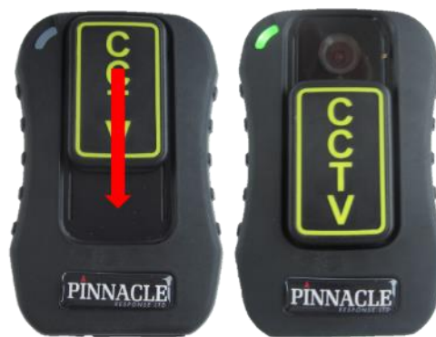
Figure 4-8. PR5 Camera Door (Power and Recording Switch)
