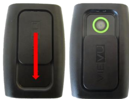
Figure 4-13. LE3 Camera Door (Power and Recording Switch)
