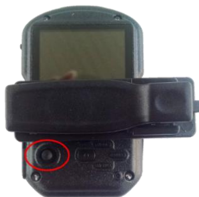
Figure 4-18. Wolfcom 3 rd Eye Police Body Camera Toggle Joystick
