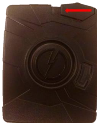
Figure 4-5. Axon Flex Power Switch
